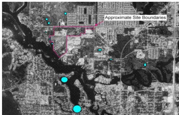
Figure 6. Aerial photo used to identify large paleosinkholes
