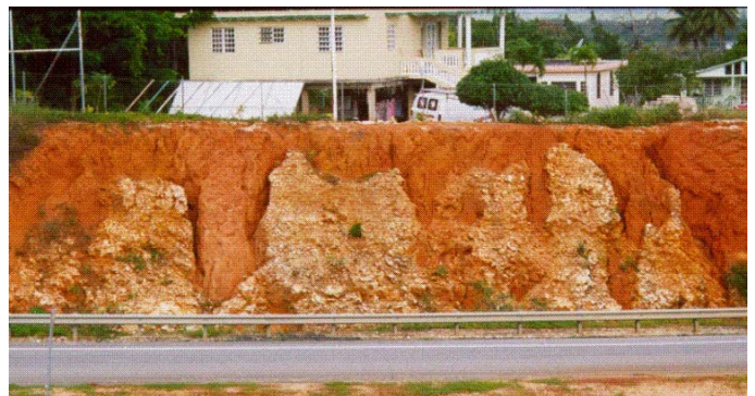
Figure 7. Highly weathered limestone exhibiting a cutter-pinnacle top of rock profile
