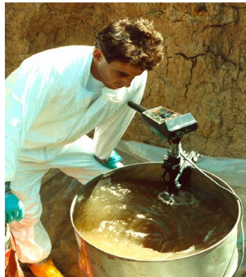
Figure 19. Mixing of dye before injection into a paleo-fracture system to assess potential flow into an underground mine in the Kansas City Area
